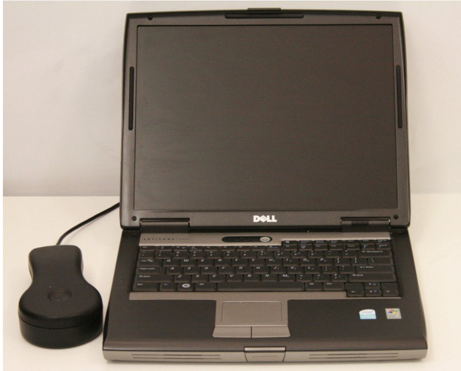
Figure 4: The NeuroPace ® Programmer and wand are used to communicate with the RNS ® Neurostimulator.
