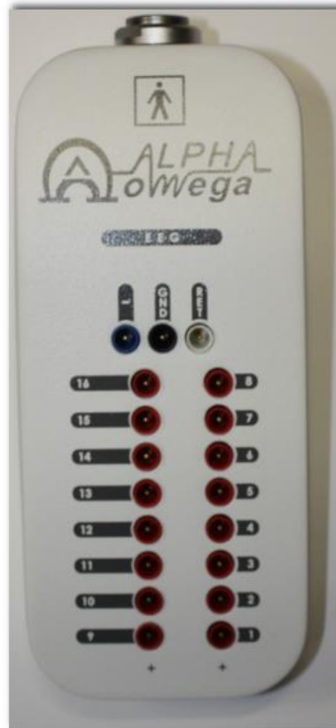
Figure 21: EEG Headbox Module
