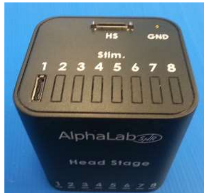
Figure 980 - Grounding input on the Headstage
