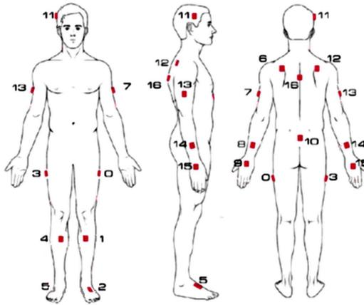
Fig. 6. The position of the IMU sensors.
